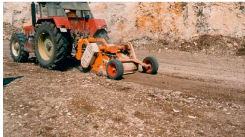
Figure 18: Stone mill for the preparation of soil
